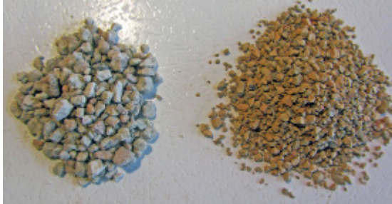
Pumice (left) and turface (right) are two more aggregate products used to increase soil drainage.
